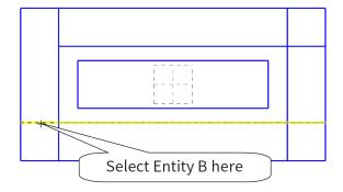
Note: Another way to remove the segments is to hold down the left mouse button and dragging the cursor across the entity.
