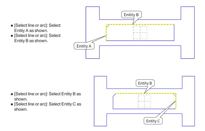
Note: Similar with divide you can also hold down the left mouse and drag it above the two entities at the corner that has to be chamfered.
