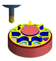
11. Convert the graphical toolpath information into machine code by Post Processing and sending it to the CNC machine.
